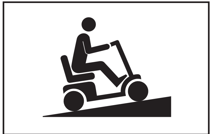
Figure 4. Increased Stability Driving Position
