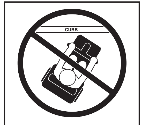
Figure 7. Incorrect Curb Approach
